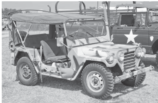
The deep-dish fender marker lights are unique to the M151A2.
