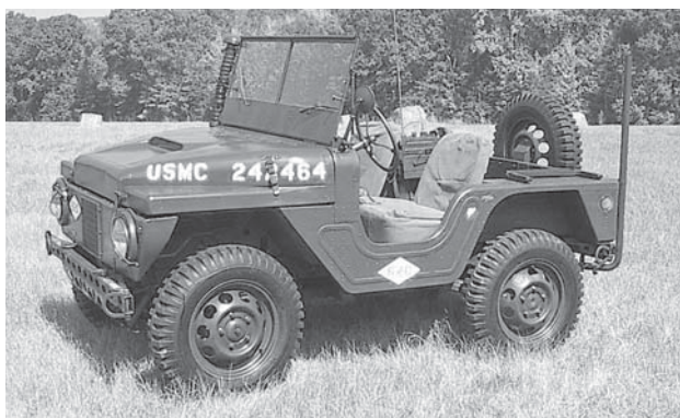
Only 1,250 M442s were made. It is six inches shorter than the M422A1.
