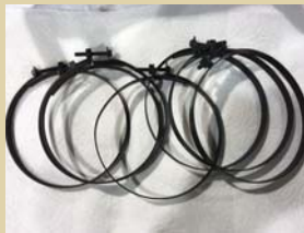
M274 Mule CV Joint Boot Clamps Install these on your mule to lessen your wheel leaks!
