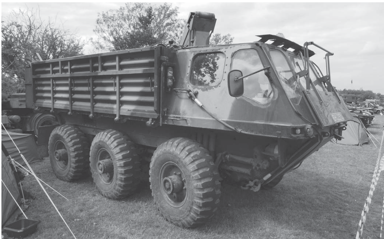
Limber/FV623 with Atlas crane in Sinsheim, Germany. Note the trio of windshield wipers — one for each of the three front windows. Stalwarts originally only had a wiper for the center window; the wipers on the outer two windows were a REME addition. Photo by Alf van Beem, Creative Commons
