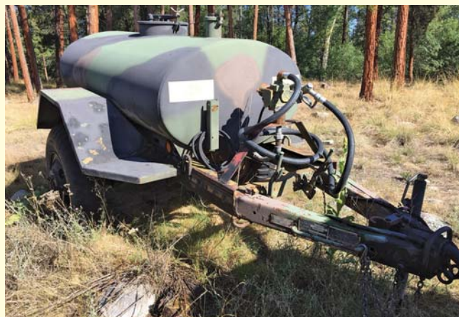
Military aluminum Fuel Tank Trailer with 12 V Transfer Pump, Hose & Nozzle
