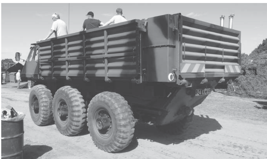
View emphasizing the Stalwart Mk 1's fold-down cargo panels. Photo courtesy of Alf van Beem, Creative Commons
