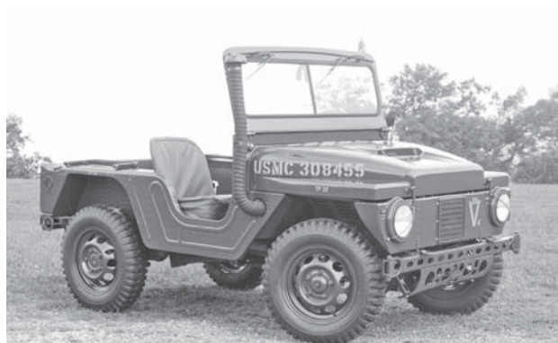
The M422A1 has an additional reinforcing rib forward of the rear tire.
